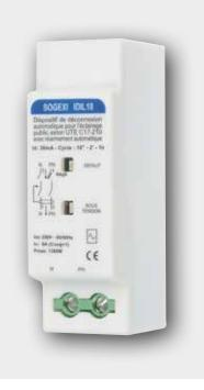
Idil primarily guarantees lighting continuity for a row of lamps should one be affected by a temporary earthing fault.
