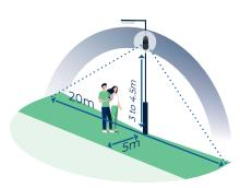
**ZONE 2:** for applications requiring a reduction at the sides of the detection zone.
