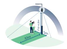
**ZONE 3:** for applications requiring a reduction of the entire detection zone.
