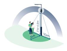
**ZONE 4:** for applications requiring a greater reduction of the entire detection zone (e.g. cycle path).
