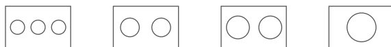
M 16 M 20 M 25 M 32 cables Ø cables Ø cables Ø cables Ø 4.5 to 10 mm 6 to 12 mm 9 to 17 mm 18 to 25 mm
