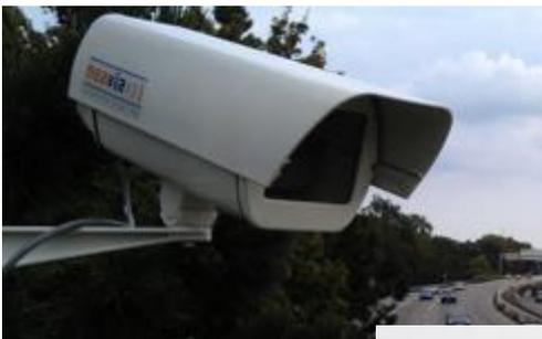
**Ecocam** is a smart, communicating, low energy consumption Webcam designed to be powered by a small solar panel.
